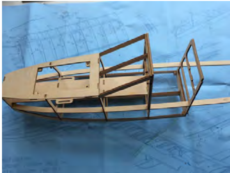
11. Glue strips A25 to the sides from the front nose former A1 back to the rear former A8.
