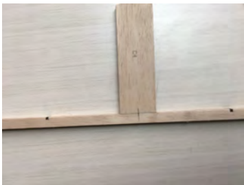
60. Glue together parts C4 and C10.
