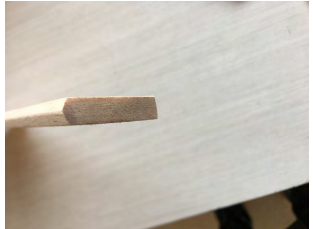
73. Sand or plane the edges of the elevators in a V to form the hinge line.
