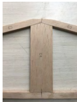
61. Add the 2 off C3 leading edge parts.
