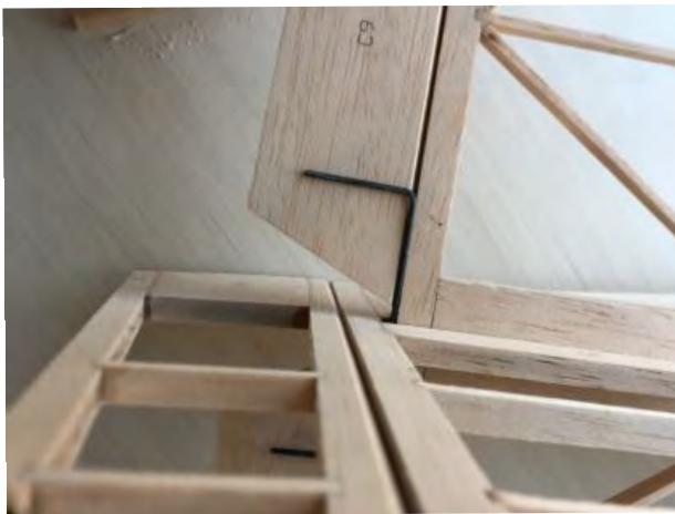
74. Hinge the elevators but do not glue the hinges in place. Pass the elevator U shaped metal joiner through the gap behind the horizontal stabilizer and position it evenly on the elevators. Mark the position ready for drilling the holes.
