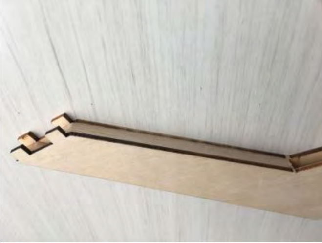
85. Construct the motor pylon using 2 off parts F2 and 2 pieces of 6x8mm hardwood.
