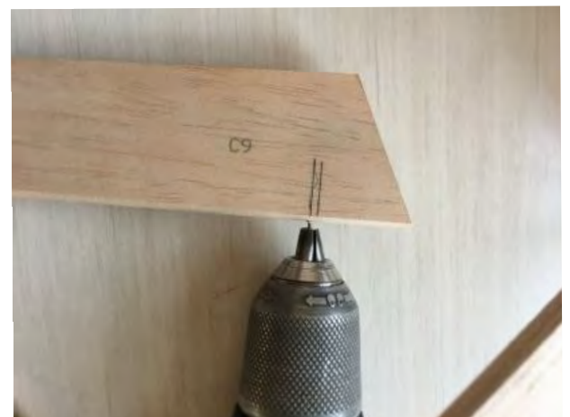
75. Drill the holes on the hinge line of the elevators to accept the U shaped metal joiner.
