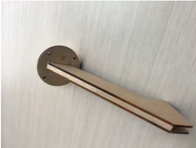
87. Glue the motor mount to the pylon.
