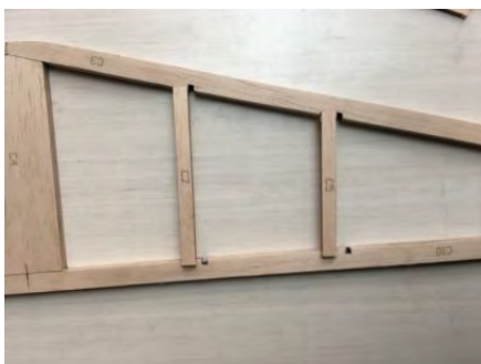
63. Add ribs C5 and C7 to both sides, glue in vertically into the slots in C3 and C10.
