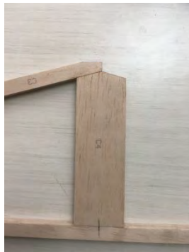
61. Add the 2 off C3 leading edge parts.
