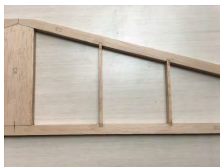
63. Add ribs C5 and C7 to both sides, glue in vertically into the slots in C3 and C10.
