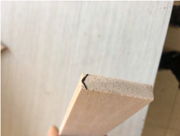
72. Mark the leading edge of the elevators with a V as shown above for the hinge line.
