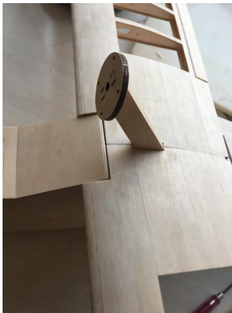
89. Glue the motor pylon securely to the wing, ensure the thrust angle is set at 5° up thrust.
