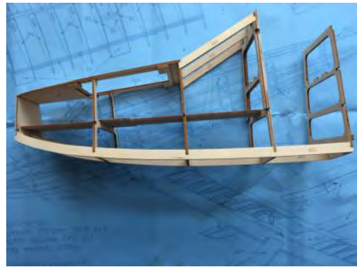
10. Glue strips A21 to front base of fuselage.
