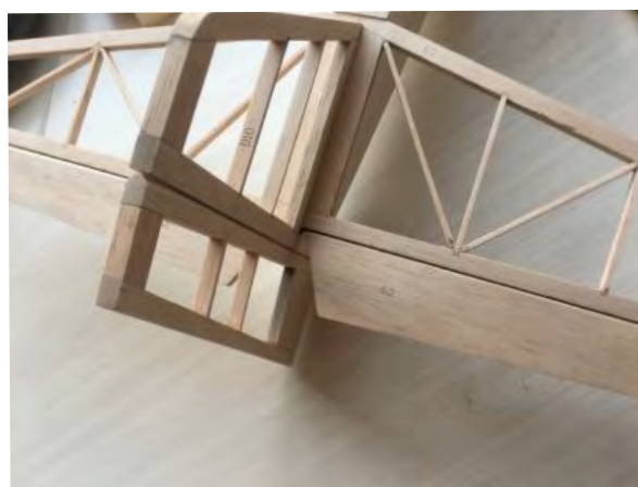
76. Replace the elevators onto the joiner and the hinges but do not glue. Fit the hinges to the rudder/vertical stabilizer but do not glue these either. The hinges will be glued in place once the model has been covered with film.
