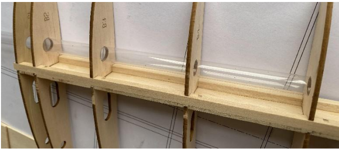
58 Preset the PVC tube(for carbon tube) in the wing.
