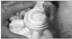
☐ 3. Cut away the prop shaft opening from the center of the Radial. Smooth the edges with a round file or drum sander.
