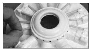
☐ 9. Insert the push pod tubes into the rocker arm covers and the crankcase as shown in the photo. They should protrude inside the Radial about 3/32" at each end of each piece. Don't worry about gluing them yet.
