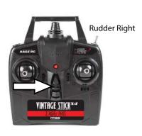
When the left stick is moved to the right of the transmitter the rudder should move right. When in flight this will yaw the tail to the left (the nose of the aircraft will move to the right).
