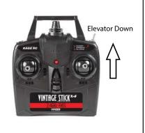
When the right stick is moved toward the top of the transmitter the elevator should move down. When in flight this will lower the nose.
