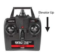
When the right stick is moved toward the bottom of the transmitter the elevator should move up. When in flight this will raise the nose.
