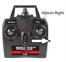
When the aileron stick is moved to the right of the transmitter the right aileron should move up and the left one move down. This will roll the wing to the right.
