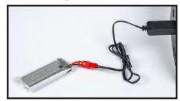
Plug the charger into a suitable 5V USB port. When the charge is complete, the red LED on the charger will light.
