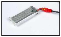
Plug the battery into the USB charge cord. Make sure that the polarity is correct by matching the red dot on the battery to the yellow dot on the connector.
