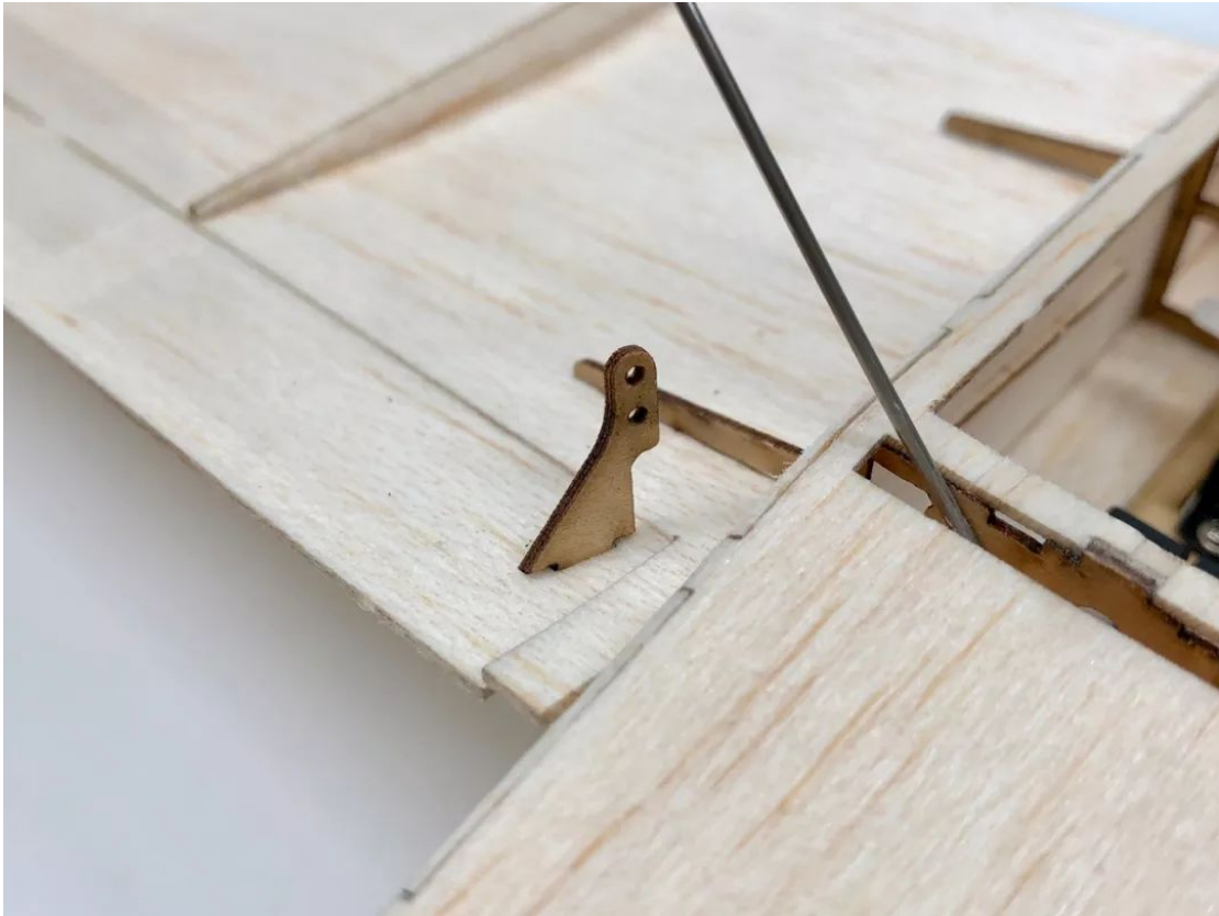
51. Installation of the control horns.
