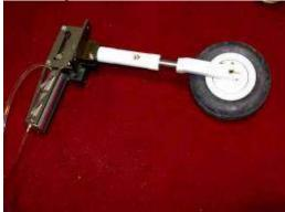
8. Trial fit the gear. You will need to cut a notch to accommodate one air nipple on the gear. Drill pilot holes for mounting screws.
