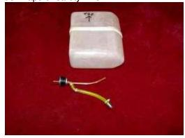
2. Carefully bend the fuel pipe to bring the clunk line more towards the center of the tank. This will allow you to use more of the fuel in the forward tank. Be sure that you do not kink the metal fuel pipes. You may have to ream out the hole in the tank slightly to fit the rubber stopper. Be sure the inside of the tank is absolutely clean of all particles before installing the stopper.
