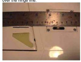
35. Drill and cut a neat, tight slot for the horn. You can drill a hole at either end, then connect the holes with your dremel tool.
