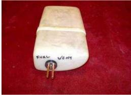
49. Add vent and fill lines to tanks. Note that the lines for both tanks must be identical in length for proper even fuel draw. Pressure tests the tanks in a sink, fix any leaks, no matter how small.
