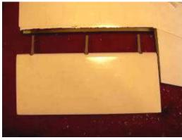
32. Using a sanding block, remove enough fiberglass to give free downward movement of the flap. Note the difference between top and bottom hinge overhangs after removal of material. Glue the hinges into the flap.
