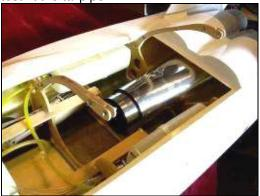
54. Install six plywood standoff blocks for the tailpipe.
