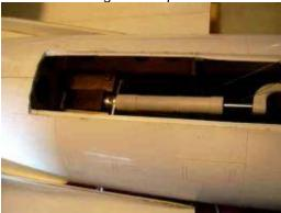
15. A standard servo is used for nose gear steering. One with metal gears is much preferred; nylon gears strip easily if you hit a bump.
