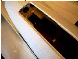
13. You will need a notch in the front former to clear the front air nipple on the nose gear.
