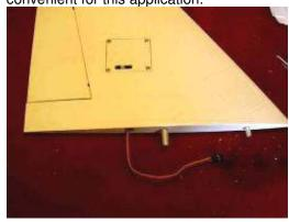
43. Drill a hole for the servo lead on the bottom of the rudder. Note there is a hole in the internal balsa rib, line the hole up with the hole in the rib.
