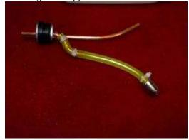
3. Attach two generous lengths of Tyron tubing to the front tank. Pressure test the tank underwater in a sink by blowing into the tubing, check for any leaks, and secure tank
