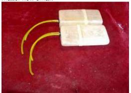
50. Install the tanks using silicone glue. Be sure to keep the glue only in places where you can get to it, in case you need to cut through the glue to remove the tanks for servicing.
