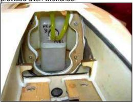
5. Two smaller bolts secure the fuse on the sides. Allen wrenches are provided in the kit. Be sure to use the correct length bolts for the side screws, otherwise they will protrude into
