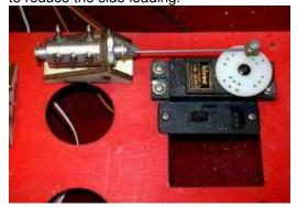
22. Install air filler valves from the bottom of the tray, and add two y-connectors and tubing as shown, to the air selector valves on the top of the radio tray. One line on each Y goes forward to your air tanks, the other lines go up to the forward nipple on the brake valve and the center nipple on the retract valve. The forward two nipples on the retract valve are for nose and mains up lines, the rear for nose and mains down. The remaining nipple on the brake valve gets the brake line.
