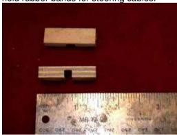
17. Connect up the steering wires with the gear in the down position. They do not need to be tight, or they will keep the gear from locking down, but they should not be slack. Install the plywood blocks. Use light rubber bands, not shown, to pull the steering cables out of the way so they do not get tangled on anything when the gear retracts.
