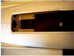
14. Install nose gear with provided screws.
