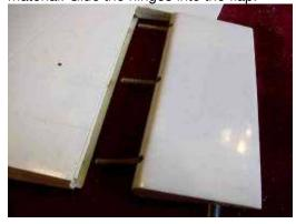
33. Glue the hinges into the wing, making sure you have enough downward movement of the flap. Note wing is upside down in the picture, you are looking at the bottom of the
