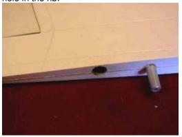
44. Work the servo lead through the hole you made and install the servo and door with four screws.
