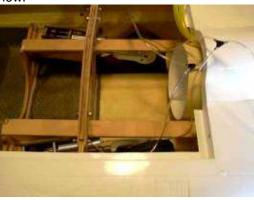
12. Remove any excess glue at the rear of the nose gear mount, remove the rear lip for the gear door as required to place the main gear and drill pilot holes.
