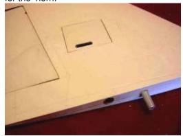
27. You can do the slots in both left and right servo doors if you flip one over and stack them together, then drill and cut.
