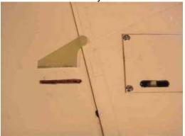
36. Install the horn with plenty of epoxy. Note that the bottom edge has a row of holes for extra mechanical grip by the glue. Make sure the holes are well filled with glue, and make sure the horn dries perpendicular to the surface.
