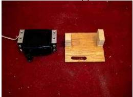
30. Mount the servo and door using four screws, not provided in the kit.
