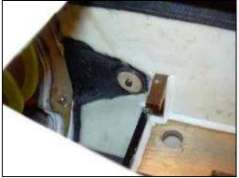
6.Remove the radio tray, held in by four screws.
