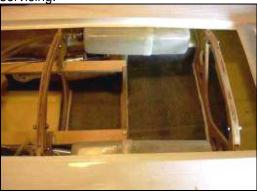
51. Add a t-fitting and a section of tubing to the main tank fill lines and run the line to the vent of the forward tank.
