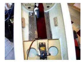
18. Connect the three sets of air lines with Y-connectors, one set for up on the mains, one set for down, and one for brakes, then run air lines forward into the nose area. Keep the lines of equal length, or both brakes will not apply equally, and both retracts will not come up simultaneously.
