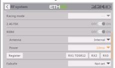
The internal RF Module can offer multiple RF power options which can achieve a further controlling range
