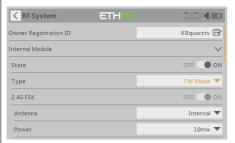
Then turn the state of Internal RF to On. Set the binding mode for the Internal RF module corresponding to the receiver (ACCST D16, ACCESS, TW, TD).
