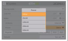
Open the Power menu bar and select the desired power level according to usage.
