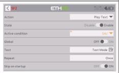
Step 2: Enable the function, and set up an "Active Condition" for it.
