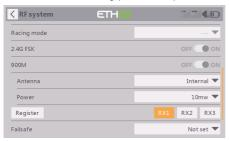
Move the cursor to RX1 [BIND], press it and repower the receiver.
