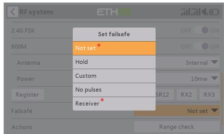
**\*Note:** In this mode after the signal is lost, the receiver will execute the failsafe state last saved by the receiver in other failsafe modes and work in the "Hold Mode" working way.
