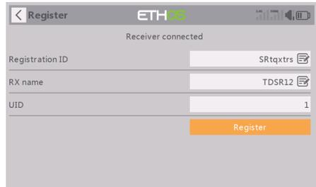
When the "RX Connected" page pops up, press the [REGISTER] to complete the Registration procedure and then power the receiver off. (The system automatically assigns the receiver a UID differently in the same model when you have several receivers to bind at the same time.)
