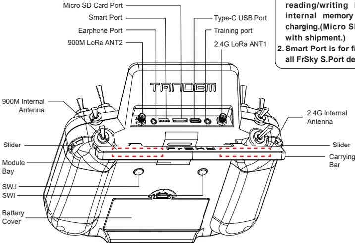
1. USB port is for system upgrading, reading/writing Micro SD cards and internal memory of radio contents and charging. (Micro SD card is not provided with shipment.)
