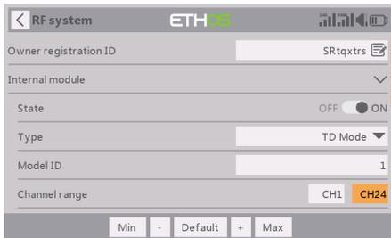
The internal RF module supports 24 channels (CH1-8 / CH1-16 / CH1-24).
