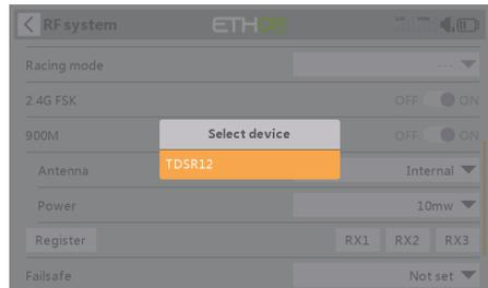
Click the RX to complete the binding after the receiver window pops up, the system will confirm "Bind succeed".
