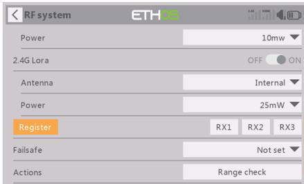
For TW Mode as an example, select the Set [Register] for getting the radio into Registration status in the RF System-Internal Module tool, then press the button on the receiver and power the receiver on.
