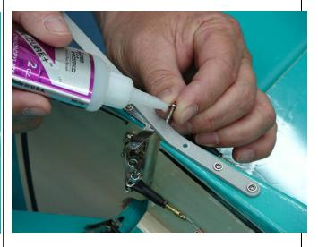
7. Mount the tail wheel strut using three wood screws.
