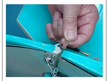
3. Apply a drop of thick CA to the mounting screws before inserting into the tiller mounting holes.
