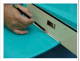
15. Remove any covering on the stab saddle as shown. This will allow for maximum gluing area.
