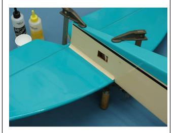
22. Allow epoxy to fully cure before removing wood clamps. It is recommended that the fuse be kept at room temperature and allowed to dry for an hour to allow epoxy to cure properly.
