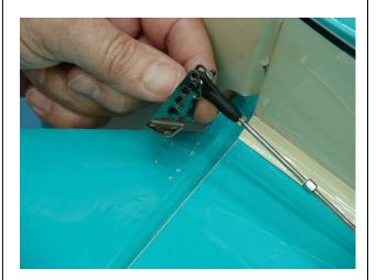
5. Use thick CA on each screw prior to installing to lock screws in place.
