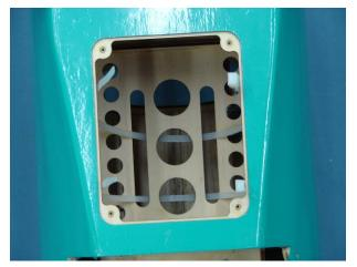
3. Install foam rubber pad for fuel tank to rest on. Foam rubber will help prevent fuel from foaming or getting air bubbles from engine vibration
