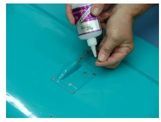
12. Install five Phillips head screws as shown. Take care not to over-tighten the screw as this can damage the servo hatch cover.
