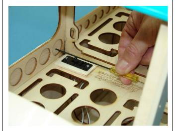
12. Using a hobby knife, puncture the location marked in the previous step. This will allow you to drill from the outside.
