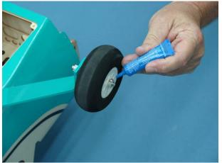
9. Slide the lock washer then the flat washer on the wheel pant mounting bolts. Use blue Loctite on the bolts before final tightening.
