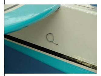
5. Pull the rudder cables from the fuse tail to the rudder servo tray. Take care not to cross the cables.
