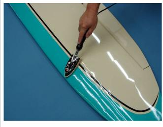
4. If bubbles persist, use a small pin to punch holes in the bubble to relieve trapped air and reheat.
