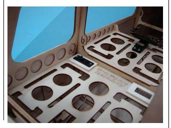
11. Use a ball driver to locate where the switch pushrod will exit the fuse. Lightly mark the wood in this area being careful not to push through the fuse side.
