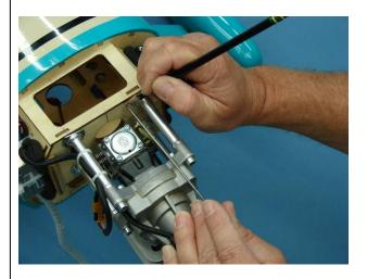
3. Use a drill bit to drill the holes for the throttle pushrod.
