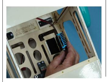
4. Slide 2 One Wrap Straps under radio tray as shown.
