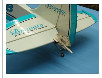
6. Aileron throw measured in degrees at widest point of the aileron.
