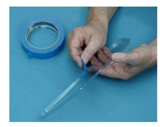
3. Stick masking tape handle to inside of window as shown. This will allow the window to be placed in the fuse cut out without smearing canopy glue.
