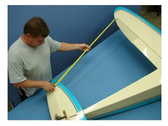
8. Making sure the airplane is completely level, sight down the elevator and ensure it is level in relation to the wing. If it is not level, it may be necessary to slightly sand the fuse on one side.
