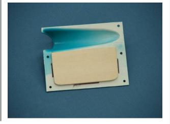
6. To ensure proper alignment, lay out the servo hatch covers as shown. There are (2) Left and (2) Right hatch covers supplied.
