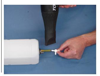
7. Install the fuel pick up and fuel filler lines to the fuel tank.
