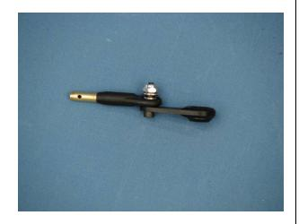
9. Placer Servo arm on servo. The servo arm should be parallel with the servo case.
