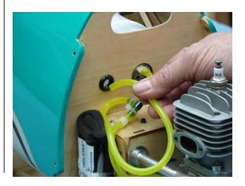
14. Feed filler line through dot and plug line into filler plug as shown.
