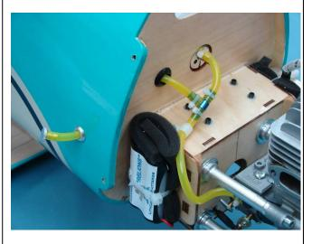
15. Feed vent line tubing through bottom of fuse. Cut off excess fuel line.
