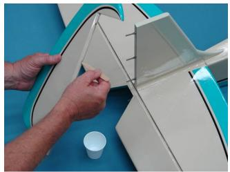
5. Carefully slide the rudder onto each hinge and against the trailing edge of the fin. Wipe away excess epoxy with alcohol wetted wipes.
