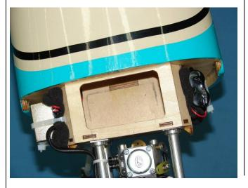
12. Place servo mounting template in motor box and align with marks made in the previous steps.
