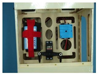
6. Mount the receiver using the same method as used for battery mounting.
