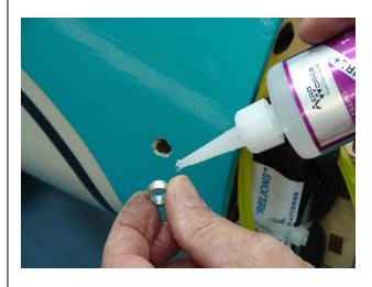
13. Drill a hole in the front fuse former and install a large grommet as shown. Pass filler line through grommet and into fuse.
