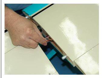
4. Slide wings away from fuse and install the CG Buddy on the wing tube and front rotation dowel as shown. The cable attachment should be on the top side of the wing. Make sure the CG Buddy is securely latched to the wing tube and dowel before moving further.
