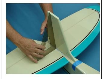
13. Place a "T" pin through the trailing edge of the vertical fin and into the stab to secure the fin while the epoxy cures.
