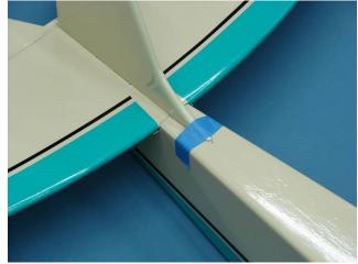
5. Use masking tape to secure the front of the
