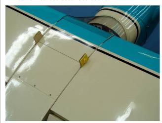
7. Wing struts must be installed when checking C.G. measuring C.G with struts not installed will effect C.G. Location.
