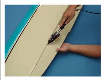
8. Use covering iron near seems and areas of exposed wood. Over heating of these areas can cause the covering to pull.
