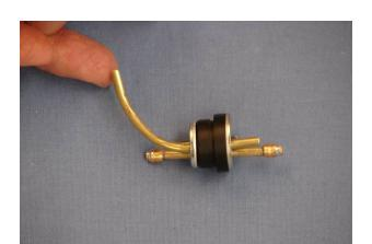
7. Install the fuel tubing and clunk. Secure the fuel tubing with nylon ties to the pick-up tube and clunk.
