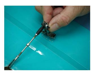
6. Use a drop of thick CA glue on each screw to prevent screws from loosening due to vibration as shown.
