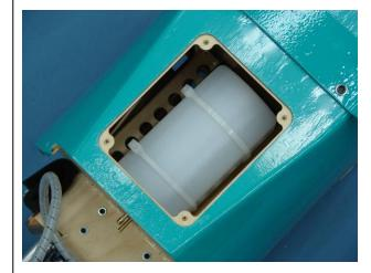
6. Install a short piece of fuel line and the fuel "T" to the fuel pick up tube.
