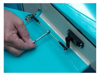
7. Finished elevator servo assembly shown below.
