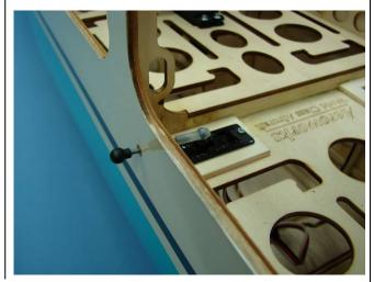
17. Using a small piece of hook and loop material, secure the Smart-Fly ignition regulator to the fuse floor.
