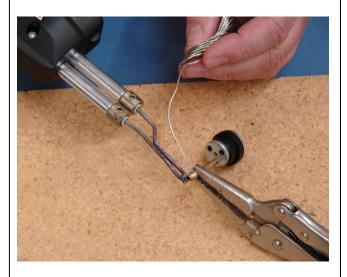
5. Final assembly of rubber fuel stopper with fuel pick up tube shown below.
