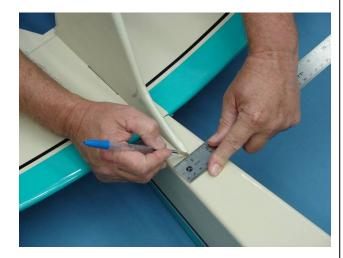
4. Use a pin to mark the location of the vertical fin on the fuse. Do not mark the stabilizer at this time.
