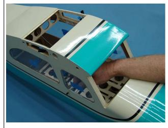
Install optional dash panel at this time. Small wood screws and double sided tape are recommended to secure dash panel.
