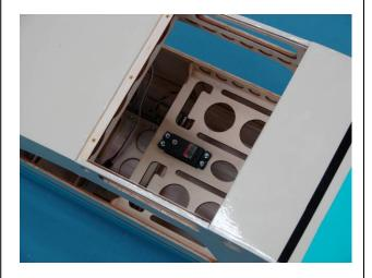
3. Feed the rudder cable through the pre installed cable exit tube in the tail of the fuse toward the front. Repeat for other side.
