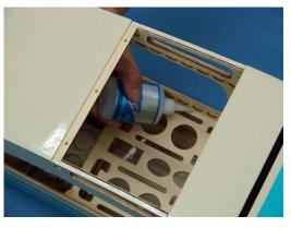
2. Apply Thin CA to all firewall joints. The firewall has already been fuel proofed and any additional fuel proofing is not necessary.
