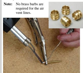
3. Assemble the fuel pick up line, rubber stopper and metal end caps. As shown below.
