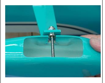
7. Install inner wheel collar. Use blue Loctite on the wheel collar set screw before final tightening.
