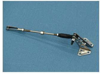
5. Align the control horns over the factory drilled holes.
