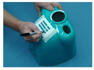
5. Remove the template and use a rotary cutting tool and sanding drum to cut out the openings in the cowl.
