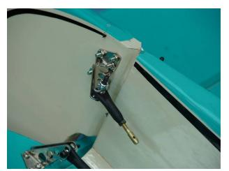
18. Final control horn installation shown below. Tighten the 2mm bolts evenly, this will prevent the control horns from crushing the rudder.
