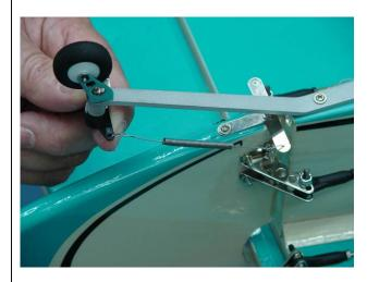
12. Bottom view of completed tail wheel installation.
