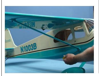
7. Secure fuse access hatch with (3) Phillips head screws as shown.
