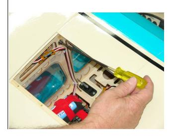
3. Attach the 18" extension to the servo lead and secure with Aeroworks Safety Clip. Ensure the connectors will not come apart from vibration or light tension.
