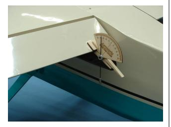
8. Elevator throw measured in inches at the widest point of the elevator
