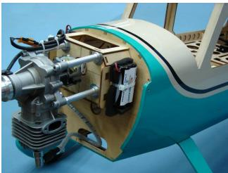
8. Using a pin vice carefully drill into the sliding portion of the switch as shown.
