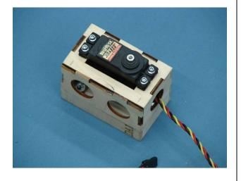
5. Place servo mounting tray inside motor box as shown.
