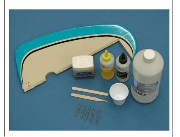
2. Prep all hinges for installation by applying Vaseline petroleum jelly or light oil to the hinge joint. This ensures no epoxy gets into the hinge during assembly.
