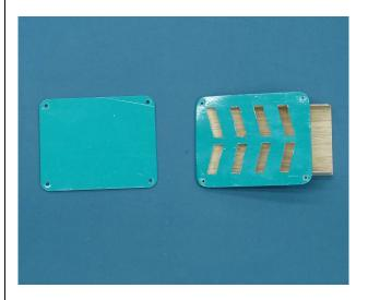
4. Place hatch into pre cut mounting location as shown. Make sure that the air scoop correctly align with the air inlet in the fuse former.
