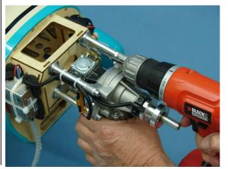
4. Install the throttle servo in the preassembled laser cut mounting tray as shown below.
