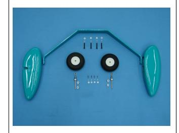
2. The tapered edge of the landing gear goes to the back of the airplane.
