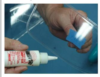
5. Place window in fuse cutout from inside fuse cabin as shown. Allow glue to full cure before removing masking tape.
