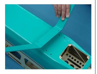
3. Attach the landing gear with bolt and flat washer. Use a drop of blue Loctite on landing gear bolts before attaching the landing gear.
