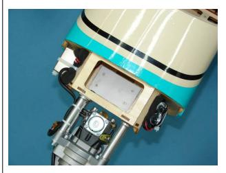
14. Drill all four mounting holes as shown. Use caution when drilling, drilling to fast may cause plywood to splinter around mounting hole.
