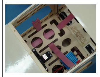
5. Install battery using foam padding and securely tighten one wrap straps as shown.
