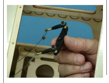
15. Assemble the ball links between the control horns as shown. Secure with nylon lock nut.
