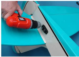
7. Install servo with servo mounting screws.
