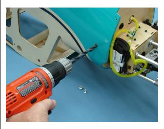
12. Use thick CA to secure fuel dot in fuse.
